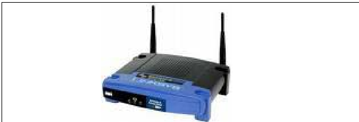
Figure 7-2. Wireless Access Point
